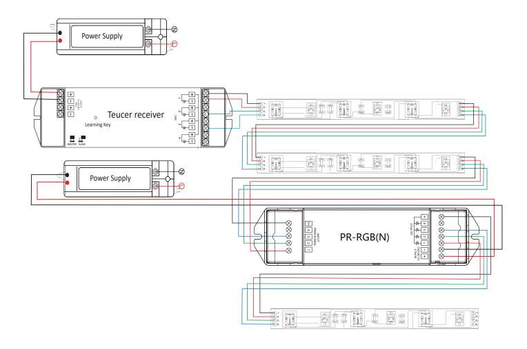
When wiring the decoders, it is important to make sure the total wattage of the LED strips does not exceed the maximum rated wattage per channel of the decoder. Each channel is rated at 5A, so the maximum wattage per channel is 24x5A=120w.
